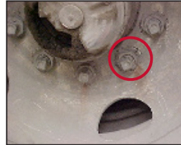
Bolt hole crack
