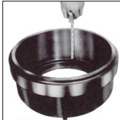
Width of braking surface
